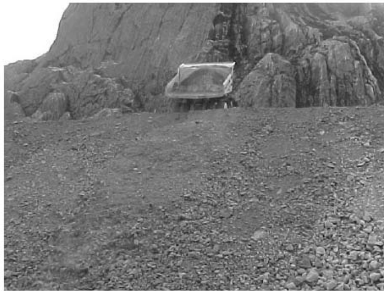
Figure 1. Gravity segregation and resulting interbedded structure in waste rock dumps.
